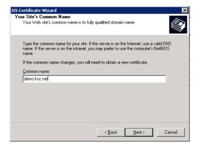
Remark: Common name is the name that will be certified by CA (Certificate Authority) as the site that is registered to the certificate installed on that server. Usually, it is a 1:1 installation, except for the Wildcard and SAN (Subject Alternative Name) certificates that are needed to be carefully installed.
